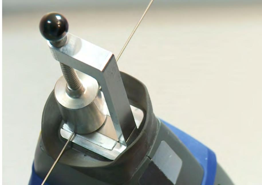
Figure 4: xSORT with small parts adapter and wire
