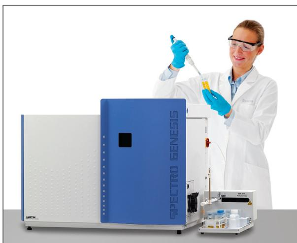
Long-term stability for an ICP-OES such as SPECTRO GENESIS is excellent. At less than 2 percent long-term instability over an 8-hour period, the instrument avoids the need for frequent recalibration.
