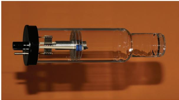
*Flame AAS, which uses a hollow cathode lamp for each element to be analyzed, has long been the hot choice for many analyses. But the increasing affordability of advanced, high-productivity ICP-OES casts a brighter light on AAS disadvantages.*
