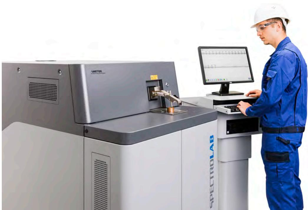
And a CMOS detector system doesn't suffer from the 80-wavelength limit that so seriously restricts how many elements a PMT-based instrument can handle. For example, one recent SPECTROLAB S installation configured the instrument to detect wavelengths emitted in 170 different analytical lines — measuring a total of 59 different elements.
