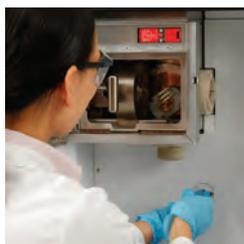
2) Rotate load coil into desired horizontal orientation
