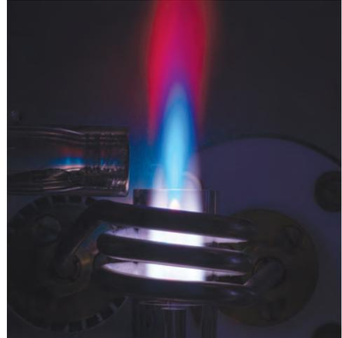
Users prefer radial models when seeking higher stability and especially higher matrix tolerance than with axial-view or dual-view models. Radial-view systems are also simpler and more robust. They require less maintenance and cleaning than their counterparts.
