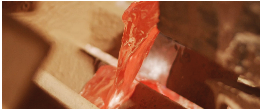
In the remelting furnace at CASS, a stream of recycled molten aluminum will be recast to the customer's precise elemental specifications — per their SPECTROMAXx analyzer. Photo courtesy of CASS. All rights reserved.
