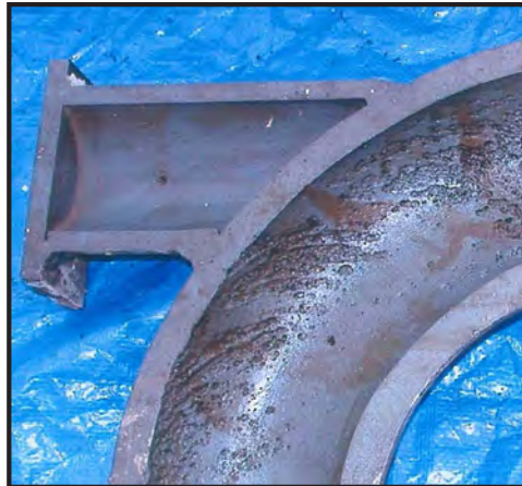
General corrosion (flow-influenced) (Photo courtesy of the Energy Institute, London)
