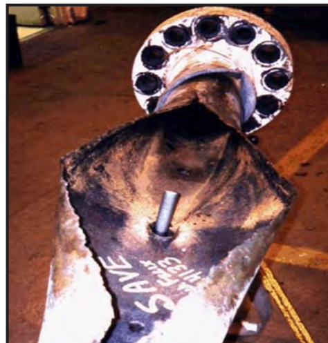
Corrosion by an acidic process chemical (scale inhibitor) (Photo courtesy of the Energy Institute, London)
