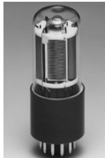
Fig 7: Typical side-window photomultiplier tube (Hamamatsu IP28)
